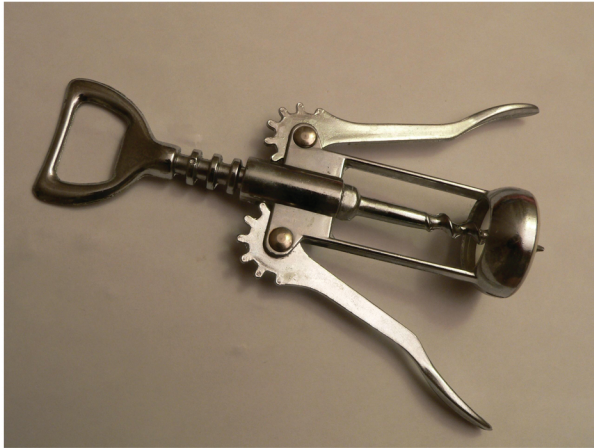
Figure 15: A double-winged lever design corkscrew
