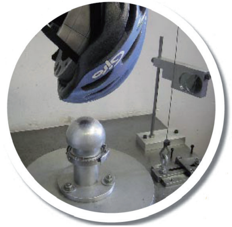
Figure 4: Evaluating protective head gear on a hemispherical anvil
